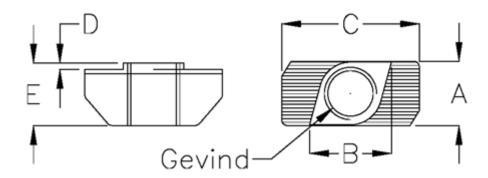
$\begin{array}{lll} A & = 9.7 \\ B & = 9.8 \\ C & = 19.5 \\ D & = 3.1 \\ E & = 8.7 \\ Thread & = M8 \\ Weight (kg) = 0.004 \end{array}$
